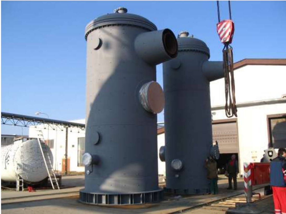
Air intercooler, air after cooler - Magnitogorsk Russia, 2007 Fluids - air / water, temperature 165/223 – 40 °C, pressure 1,3 – 11 bar(g), 1.4301, Al, P265GH, 27 300 kg,
