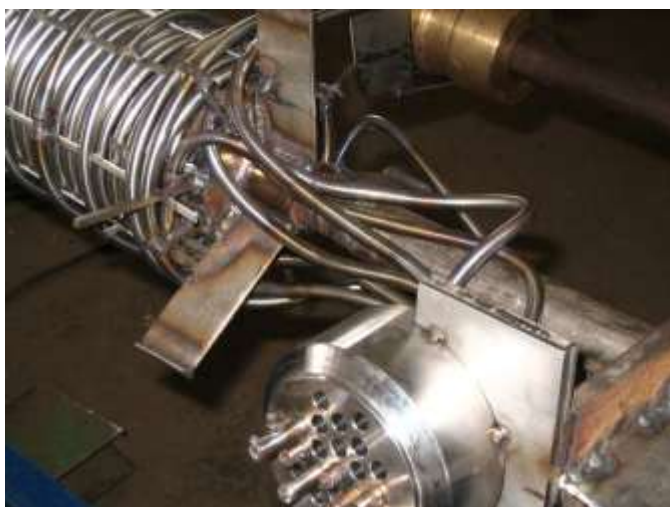
Low temperature heat exchanger, Chart Inc. USA, 2010, +150/-196 °C, 220/16 bar(g), AISI 321, fluid CH 4 , N 2 , acc. to ASME Code Sect. VIII Div.1
