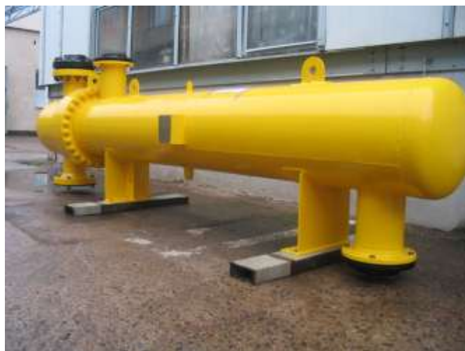
Bypass cooler Kremencuk, Ukraine, 2011, Fluids hydrogen, methane, 54/6 bar (g), 135/25 °C, 2 MW, 3 000 kg, carbon steel
