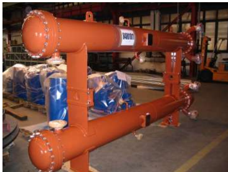
Oil / water coolers, 2000-2011, 80 – 500 kW, 90/45°C, 6-8 bar(g), stainless steel, carbon steel
