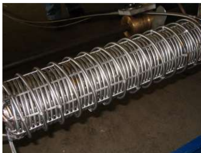
Low temperature heat exchanger, Chart Inc. USA, 2010, +150/-196 °C, 220/16 bar(g), AISI 321, fluid CH 4 , N 2 , acc. to ASME Code Sect. VIII Div.1
