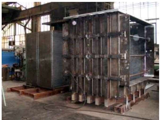
Flue gas cooler input / output chamber (Žirany SK, 2005), cooling fluid water, 4 pcs, 8105 Nm 3 /h, flue gas temperature 355/160 °C, water temperature 70/90 °C, exchanged heat 606 kW, 3 bar(g), tubes OD 44,5 mm, material carbon steel, 3200 kg
