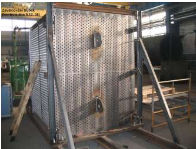
Flue gas cooler input / output chamber (Žirany SK, 2005), cooling fluid water, 4 pcs, 8105 Nm 3 /h, flue gas temperature 355/160 °C, water temperature 70/90 °C, exchanged heat 606 kW, 3 bar(g), tubes OD 44,5 mm, material carbon steel, 3200 kg
