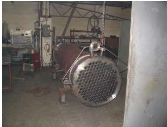
Flue gas cooler input / output chamber (Žirany SK, 2005), cooling fluid water, 4 pcs, 8105 Nm 3 /h, flue gas temperature 355/160 °C, water temperature 70/90 °C, exchanged heat 606 kW, 3 bar(g), tubes OD 44,5 mm, material carbon steel, 3200 kg
