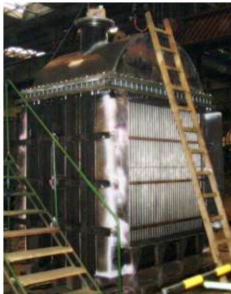
Water / air cooler, Enakijevo Ukraine 2008, air temperature 160/45 °C, material 1.4301, Al, carbon steel, 18 000 kg
