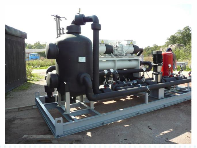
» Nitrogen Recuperation Unit (Cooling, Drying, Heating), Chart Ferox, CZ
